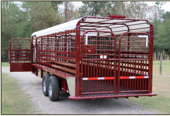
Heavy Duty Butterfly Cattle Gates With 2x4 Tubing Frame and Pipe Latch. Sliding tailgate also available.
