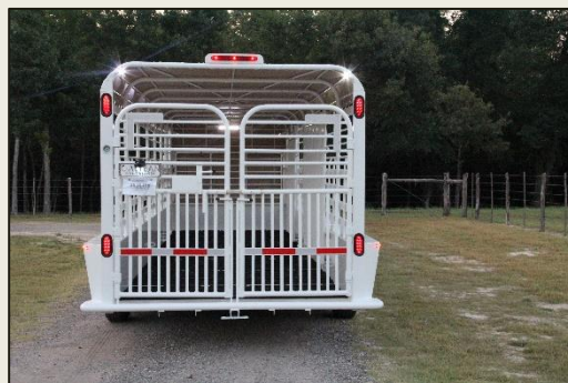
Optional LED Load Lights with toggle switch in 2x4 post
