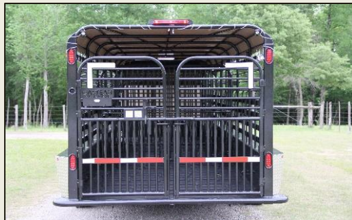
Heavy Duty 2x4 Tubing Uprights with Quad Tail Lights (Reverse lights also available)
