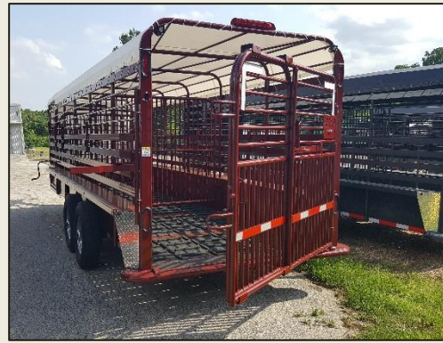
Heavy Duty Butterfly Cattle Gates With 2x4 Tubing Frame and Pipe Latch. Sliding tailgate also available.
